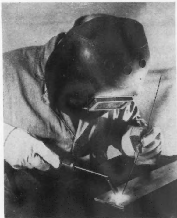
FIG. 2 —Electrode holder is inclined slightly away from the direction of travel, and filler rod is added by alternately inserting and withdrawing it from the molten pool.
